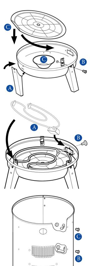
D. Align Handle Bracket (13) over one pair of holes near the top of the Body Assembly. Insert a  $10-24 \times 3/8$ " bolt (2) through each hole in the Bracket then through the Body. Fasten in place with a Lock Nut and tighten. Repeat for Handle Bracket on opposite side of Body Assembly.
